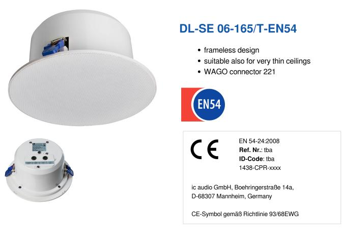
Inspired by the look of contemporary LED lights, the frameless design of the new 6W loudspeakers has all the makings of an instant classic. The 6W powered speaker is equipped with a 165mm full-range loudspeaker and a 100V transformer with 3 power adjustments. The powder coated metal in RAL 9016 guarantees long-term stability. For additional reliability the speaker is impregnated against wetness.
